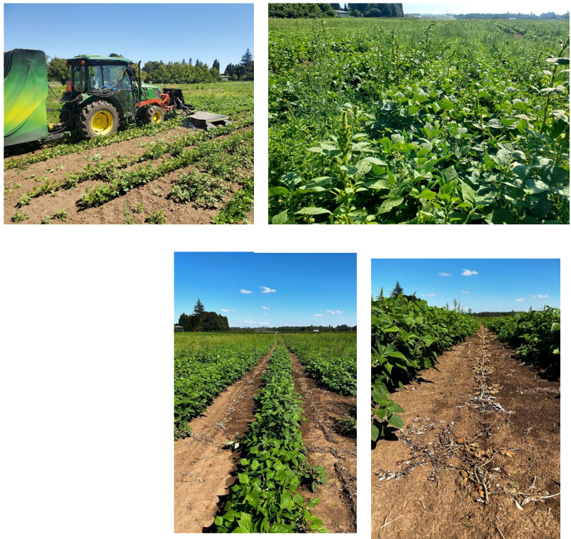
Figure 1. Top left , the Zasso (EH 30 Thor) currently available at OSU. Top right , the nontreated snap beans check 14 days after treatment. Bottom left , an electric weed control application within snap beans 14 days after treatment. Bottom right shows crop row removed by current equipment.
