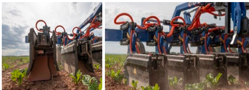
Figure 2. Electric weed control (EWC) interrow applicator in sugar beets developed by Zasso. Photo obtained from website.
