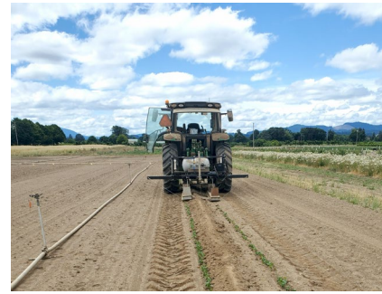
Figure 2. Two-row flamer used in the study to apply over the crop rows in trial 1. The snap beans emerged too early and were larger than the weeds at time of application leading to significant injury on the beans.
