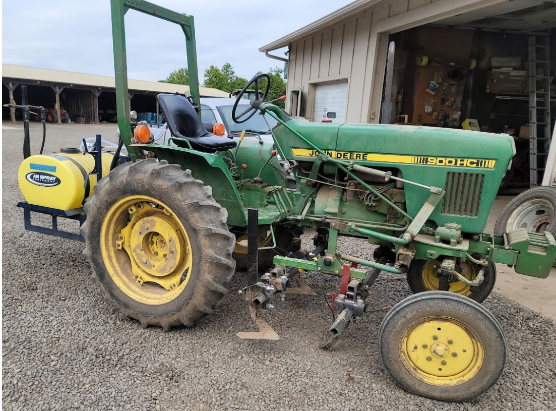
Figure 1. Tractor and equipment used for liquid N sidedress application for a supersweet corn fertility trial grown at the OSU Vegetable Research Farm in 2023.
